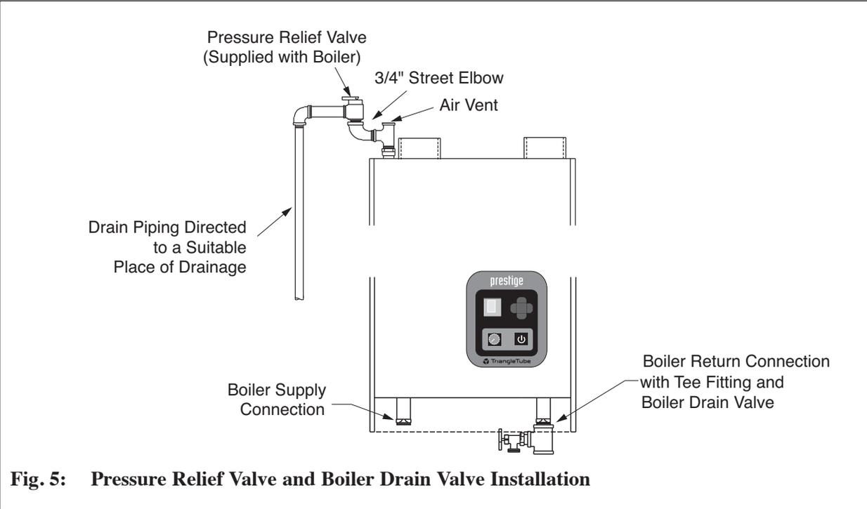
**Fig. 5: Pressure Relief Valve and Boiler Drain Valve Installation**
