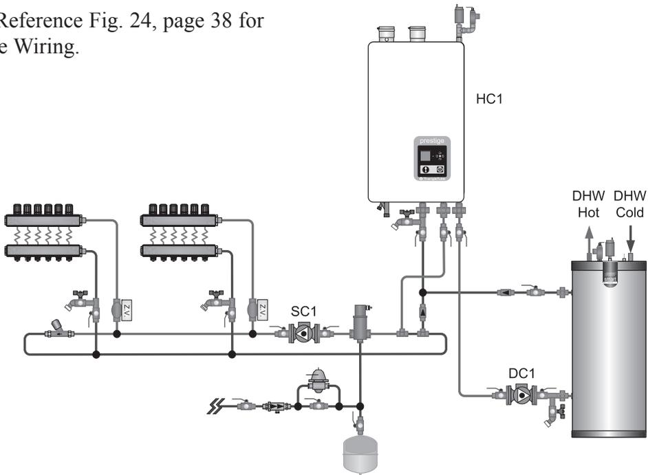
**Fig. 10: System Piping - Zoning with Zone Valves**
