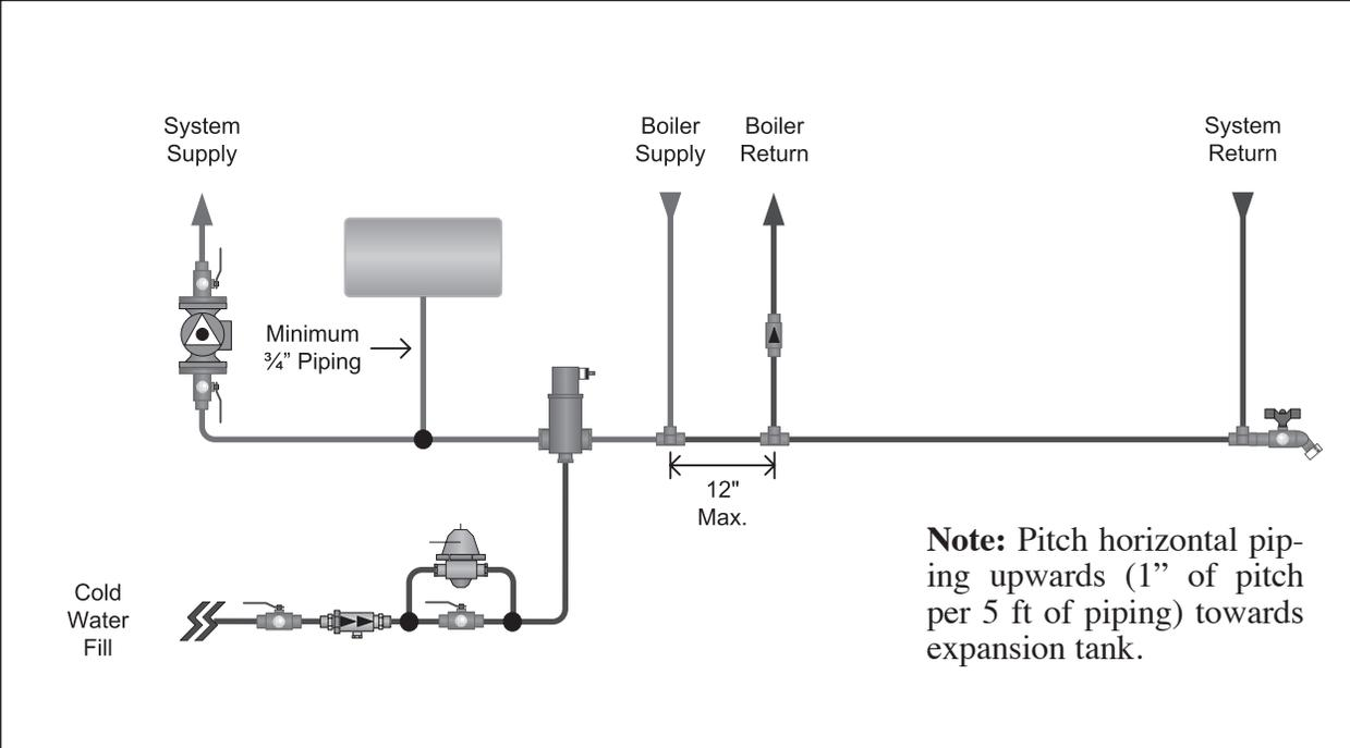
Fig. 8 : Near Boiler Piping - Closed Type Expansion Tank
