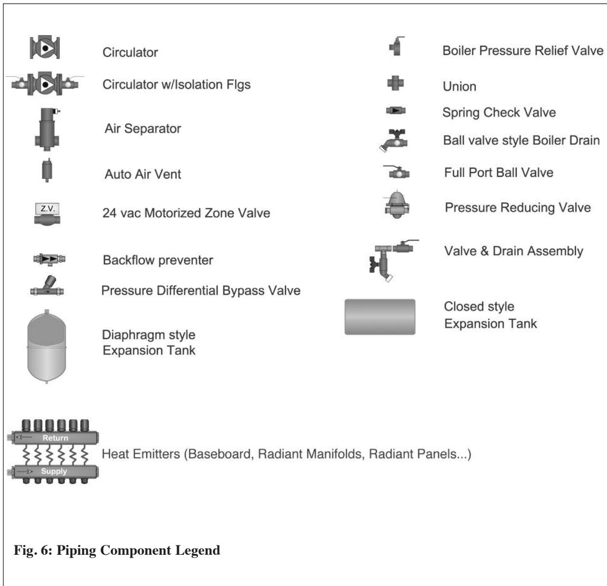
**Fig. 6: Piping Component Legend**
