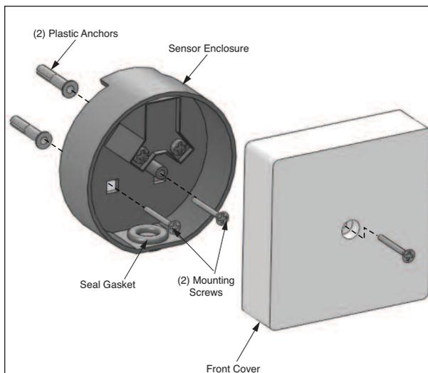
Fig. 32: Sensor Enclosure and Components
