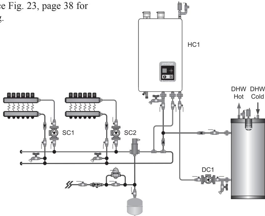
**Fig. 9: System Piping - Zoning with Zone Circulators**
