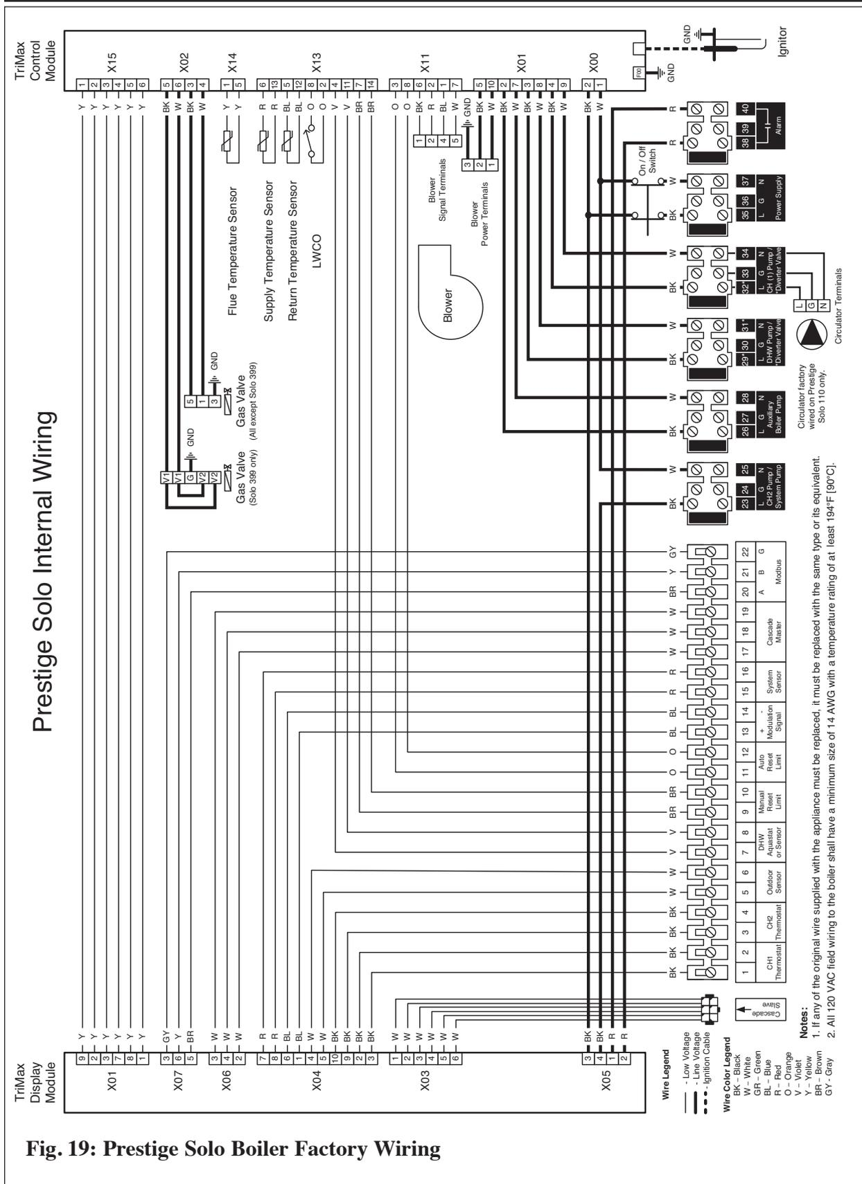
Fig. 19: Prestige Solo Boiler Factory Wiring
