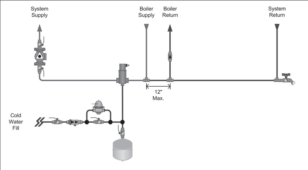
Fig. 7: Near Boiler Piping - Diaphragm Expansion Tank
