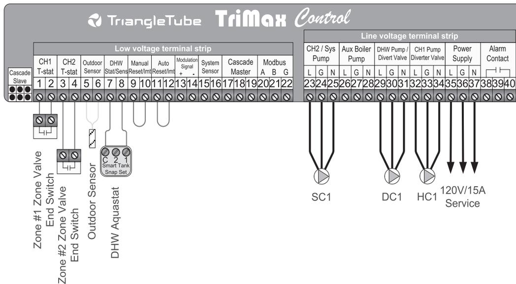
**Fig. 24: Prestige Wiring - Zoning with Zone Valves**
