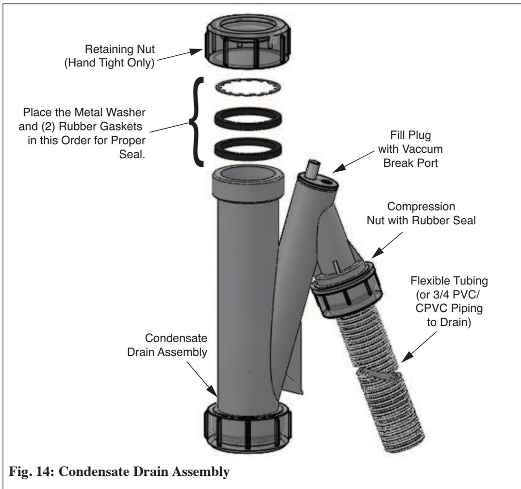
**Fig. 14: Condensate Drain Assembly**
