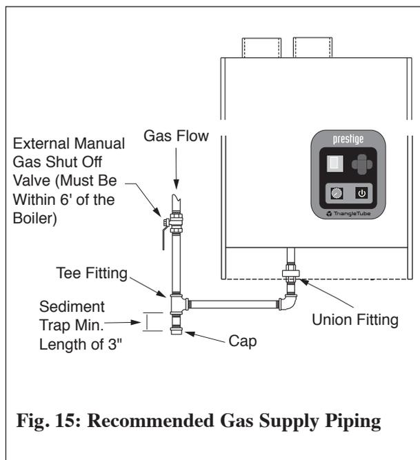
**Fig. 15: Recommended Gas Supply Piping**
